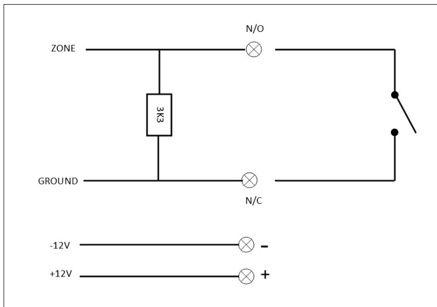
Figure 3 Serial EOL with Normally Closed Contact
